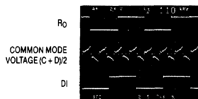
Figure 7. System Common Mode Voltage @ 110kHz
